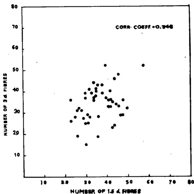
**Fig. 2.** Relation between number of 1.5-den and 3-den fibers, denier-difference blend (No. 3).
