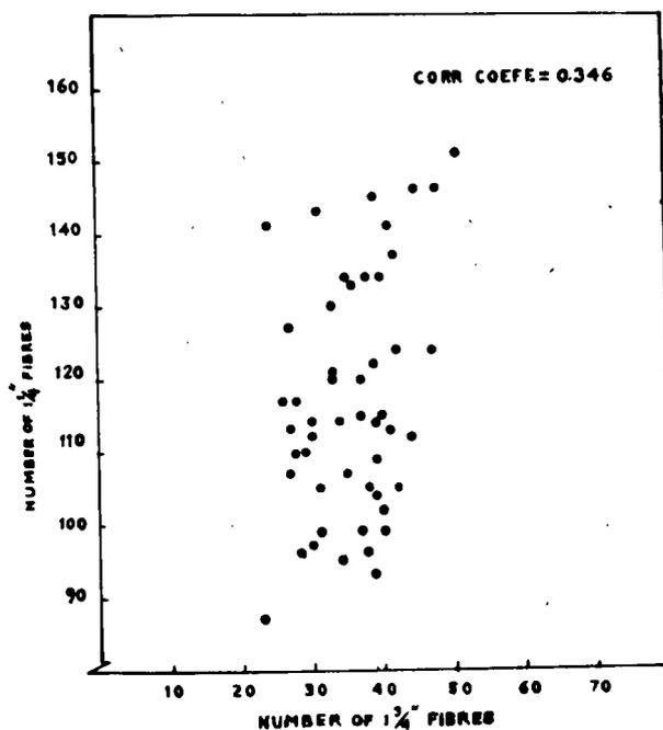
**Fig. 3.** Relation between the number of 1 1/4-in. fibers and 1 1/2-in. fibers, length-difference blend (No. 2).
