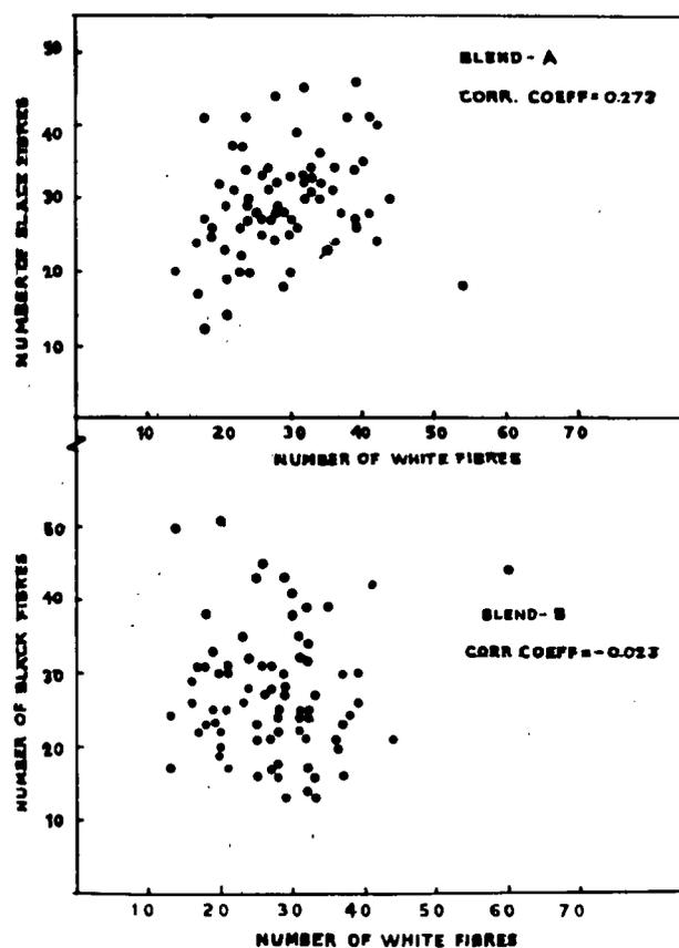
Fig. 7. Relation between the constituents in blends differing in intimacy of lateral mixing.
